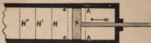
FIG. 10.—Illustrating the production of sound waves.
